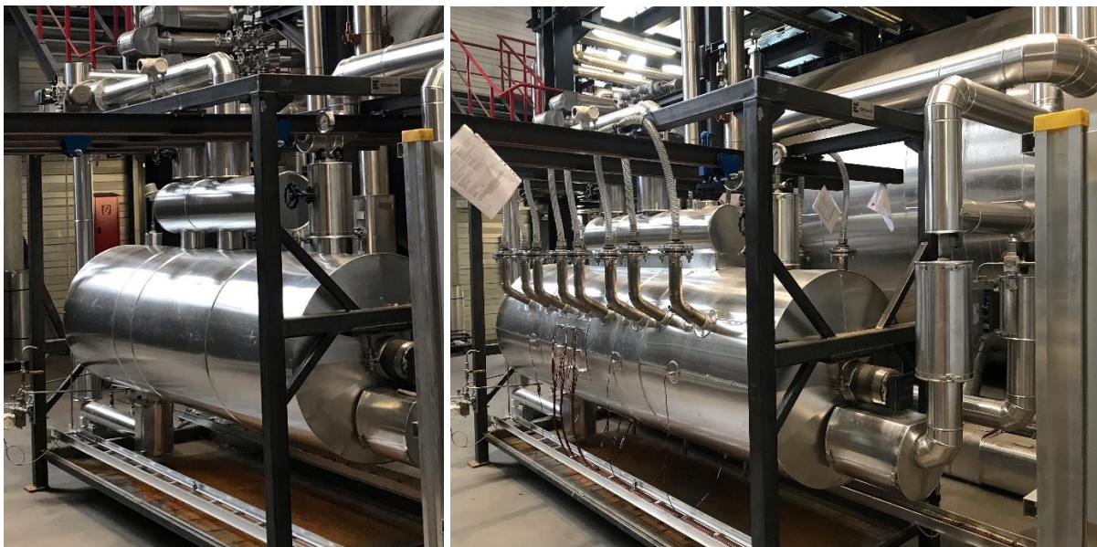
Figure 4.16: Lab scale Ruths steam storage, comparison without modules (left) and with PCM-modules (right)
