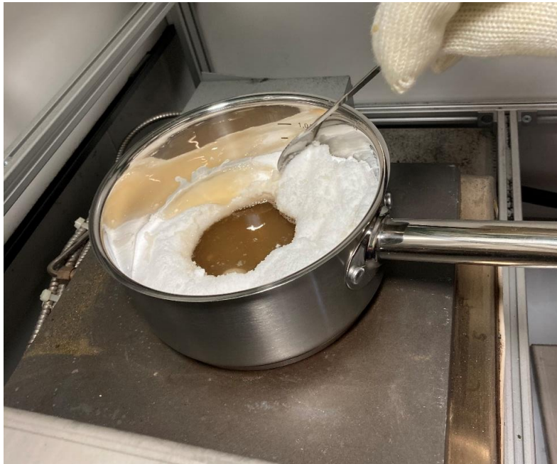
Figure 4.14: Heating process of PCM
