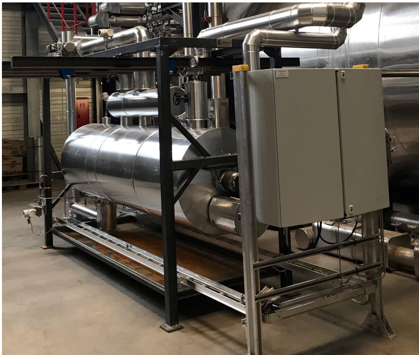
Figure 4.12: Lab scale Ruths steam storage device insulated and ready for experiments in May 2021
