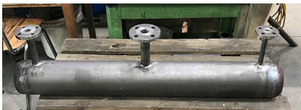
Figure 4.9: Collector under construction
