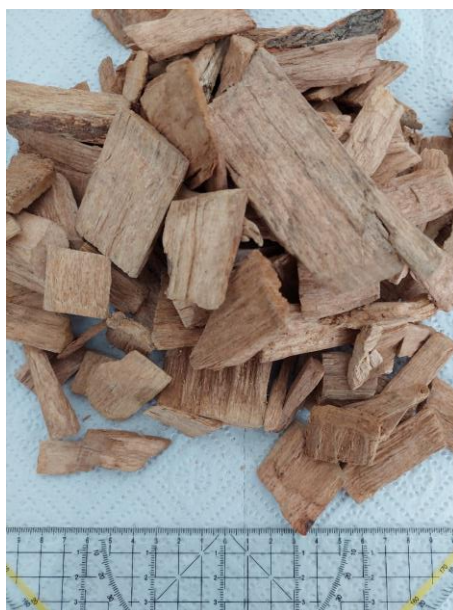
Figure 8: Beech chips used during the test runs
