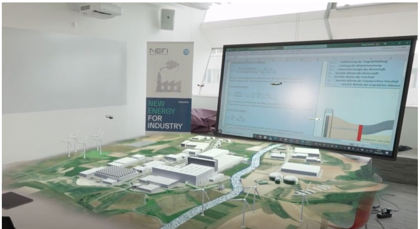
Figure 23: A dedicated tool was created by AIT allowing an immersive planning process via Augmented Reality enabling optimal technical solutions as well as facilitating social acceptance via an interactive public stakeholder dialogue. The AR tool is directly coupled with the Dymola models that can simulate the techno-economical key
