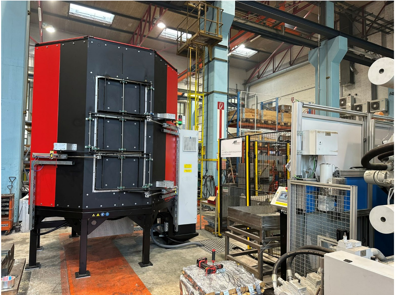
Figure 38: Installation of the solutionizing furnace the Green Foundry 4.0 demo factory at AIT LKR Ranshofen
