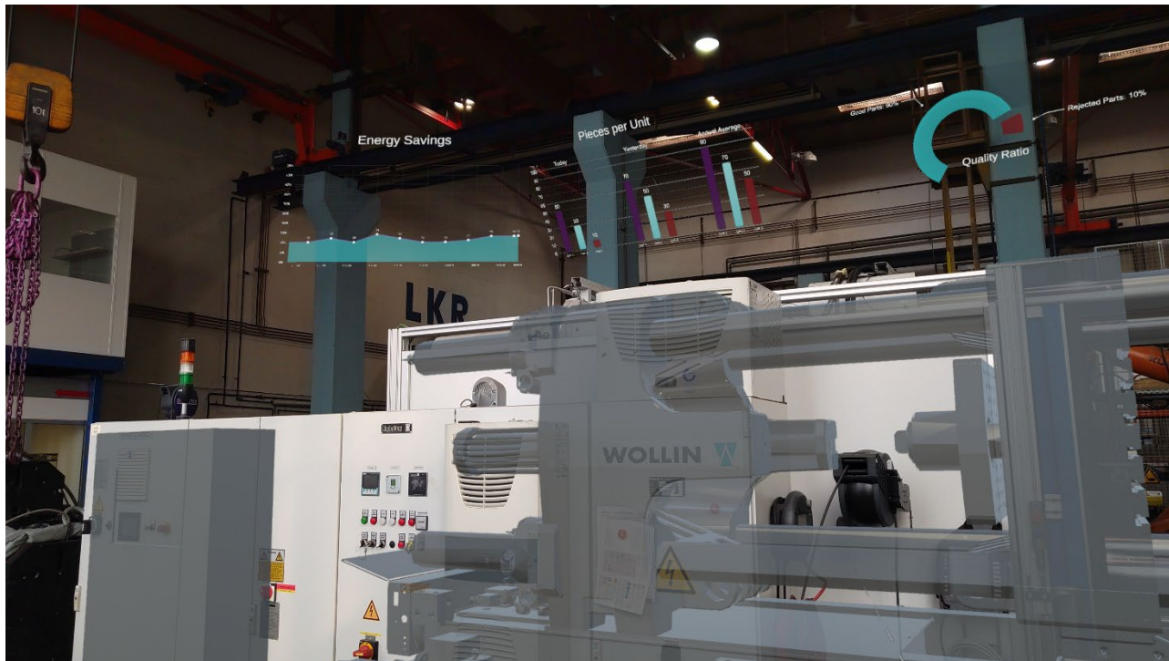
Figure 43: AR overlay of the die casting machine with live process and energy data.
