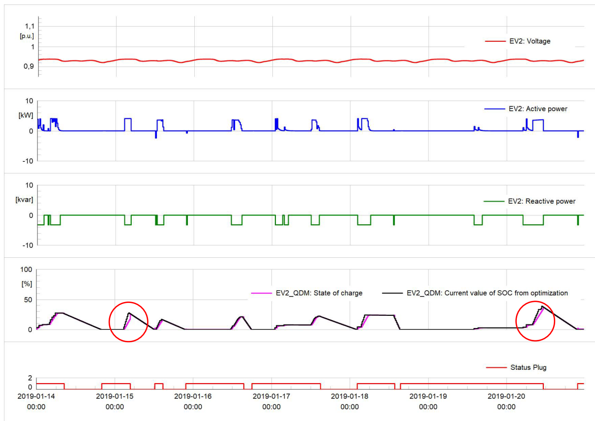
Figure 58: Realizing a schedule with P(U) control activated
