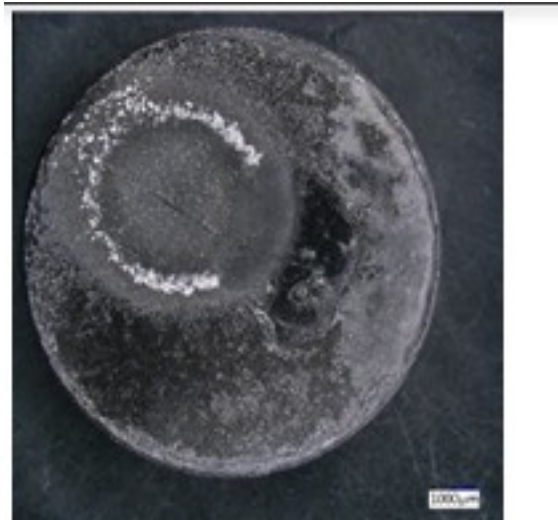
Figure 8. Reaction Zone of B disc after plasma reaction
