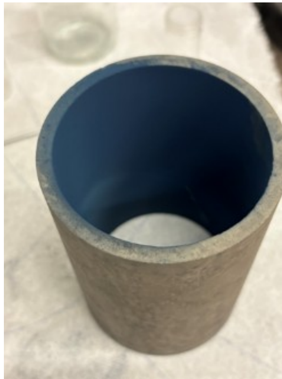
Figure 12. Tungsten suboxide coating on a Al 2 O 3 substrate ( \text{WO}_3 \rightarrow \text{WO}_{3-x} ).
