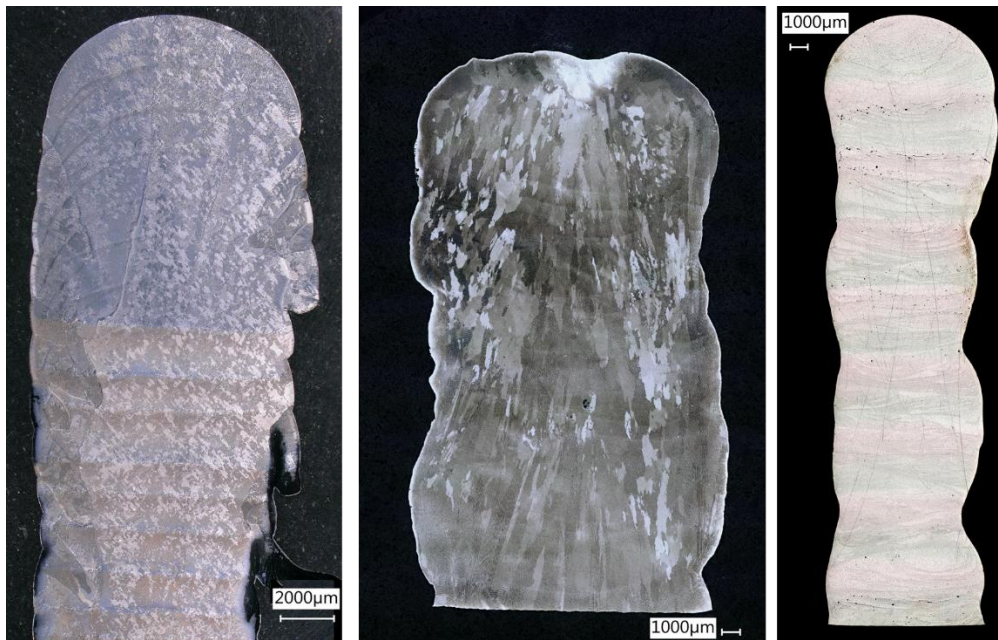
Figure 7 - Cross-sections of the non-steel alloys produced via PMD. From left to right: Ti-64, In718, AlMgSc
