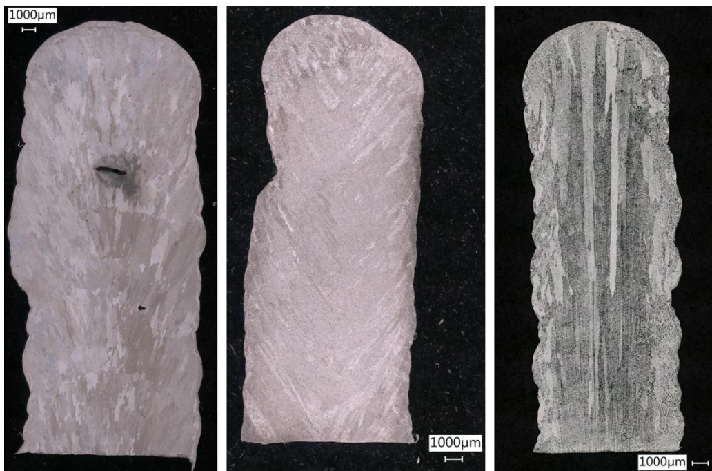
Figure 5 – Cross-sections of the steels produced via PMD. From left to right: 316L, 2209, 1.4477
