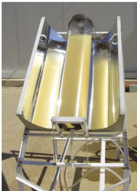
Figure 3-1: Solar disinfection reactor (SODIS) [42]
