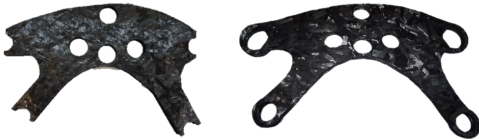
Figure 13: C-SMC preforms for the transmission cross beam: Left, with weld lines; right, without weld lines.
