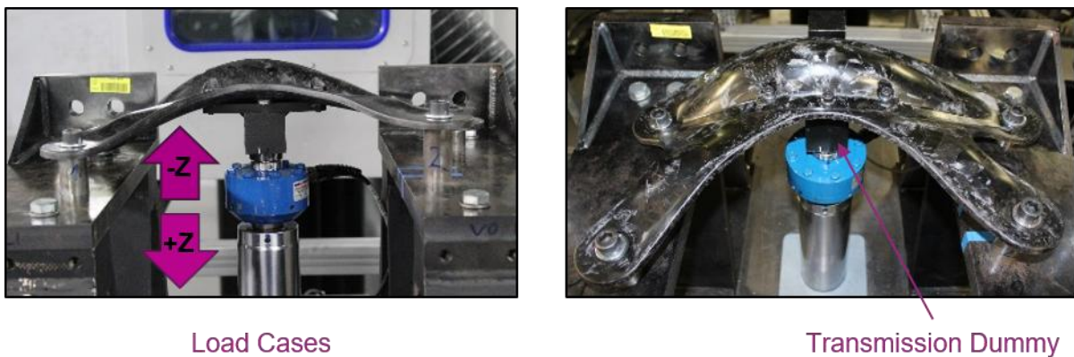
Figure 17: Component testing set-up after OEM requirements.
