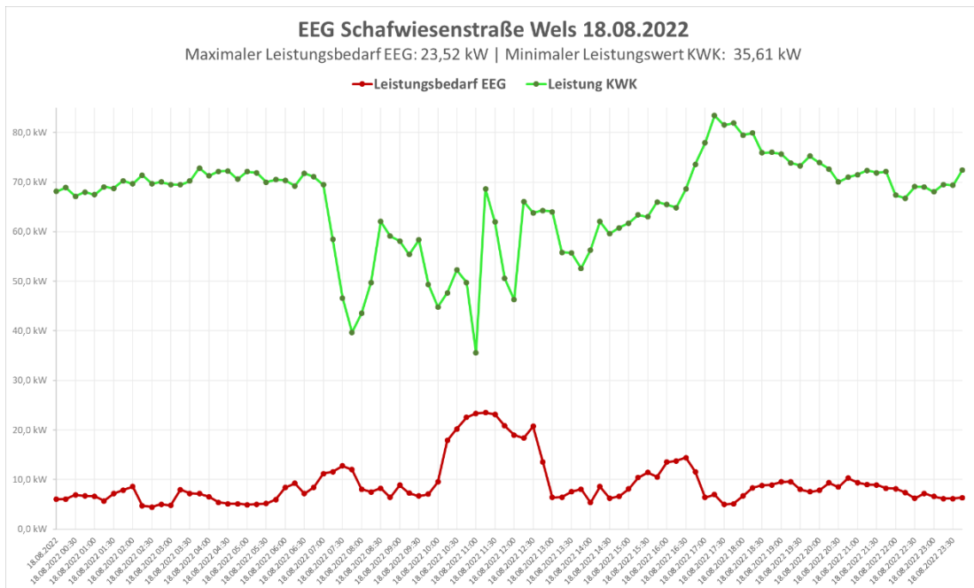
Figure 30: Course of the day (18.8.2022) of the energy production (green) and the load from the energy community (red)
