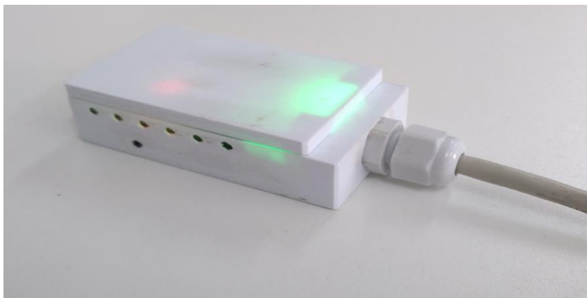
Figure 41: battery sensor platform, Gen2 with enclosure.
