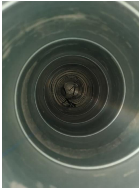
Figure 19: Experimental setup of the general advection experiments with line of sight from the injection point to the other end of the tube.
