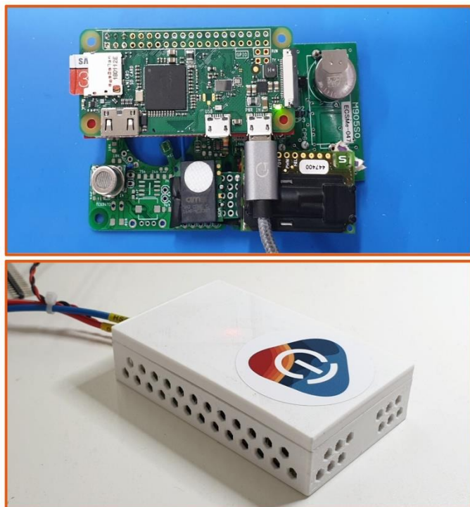
Figure 39: Battery Test box
