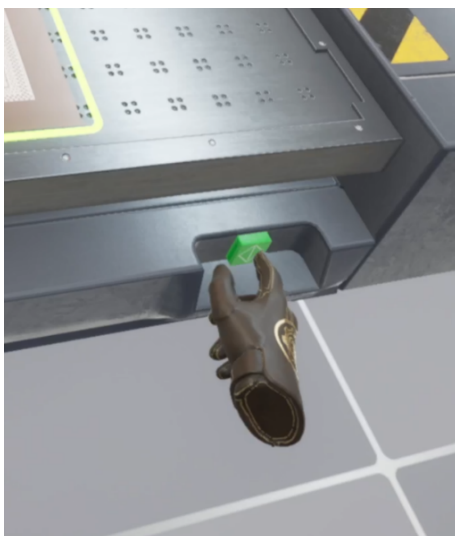
Figure 38: Change in the virtual hand pose based on the distance to the touch-interactable objects.
