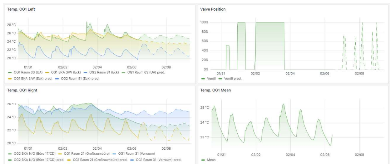
Figure 52: dashboard visualization of the predictive control in building Inffeldgasse 21B
