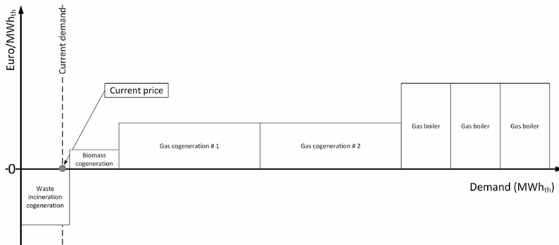
Figure 15: Order of units in the heat merit order model in an exemplary hour in the summer. To cover the total heat demand, only parts of the thermal capacity of the first unit – according to marginal costs – is utilized. Source: Moser, Puschnigg, Rodin (2020). Designing the Heat Merit Order to determine the value of industrial waste heat for district heating systems. Energy 200, 117579.
