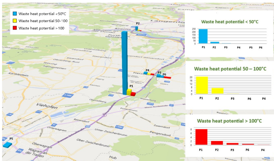
Figure 26: Waste Heat Potential Map for St.Pölten-Krems Region
