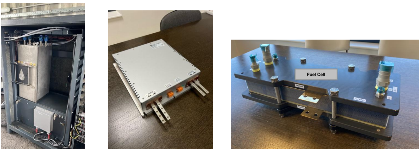
Figure 11: Further developed components of JOHANN (fuel cell (assembly in frame), DC/DC converter, partially assembled fuel cell)
