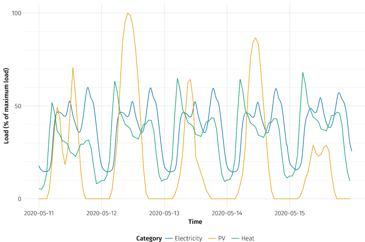
Figure 06: Normalized electricity demand, head demand and PV production profiles during five days in May 2020
